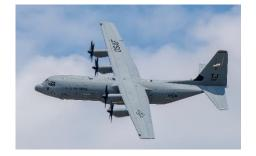
C-130J Super Hercules (Manufacturer: Lockheed Martin) General characteristics Crew: 3 (Capacity: 128 passengers or 92 airborne troops) Powerplant: 4 × Rolls-Royce AE 2100D3 turboprop Propellers: Dowty R391 6-blade composite propeller Length: 112 feet, 9 inches (34.41 meters) Height: 38 feet, 10 inches (11.61 meters) Wingspan: 132 feet, 7 inches (40.45 meters) Speed: 410 mph/356 ktas (Mach 0.58) at 22,000 feet (6,706m)
